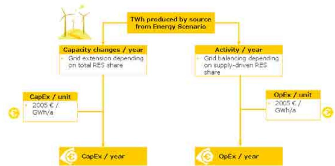
Figure 6 - 18 Approach for electricity grids.
