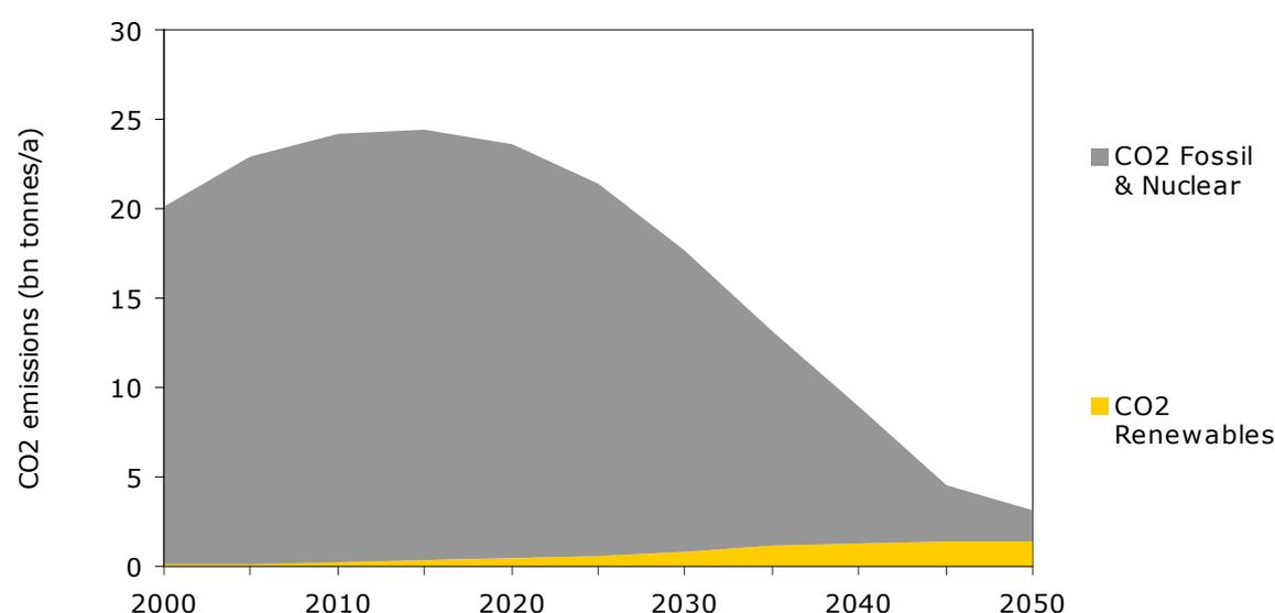
Figure 4 - 14 Global CO<sub>2</sub>-eq GHG emissions from the energy system in the Scenario.
